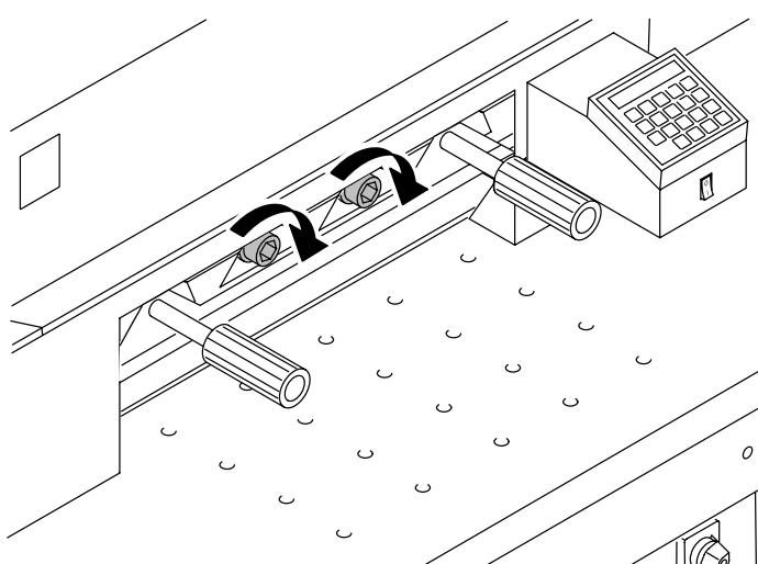
Screw in middle screws and tighten.
