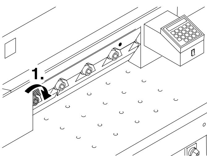
Push in the first screw on the left side and tighten.
