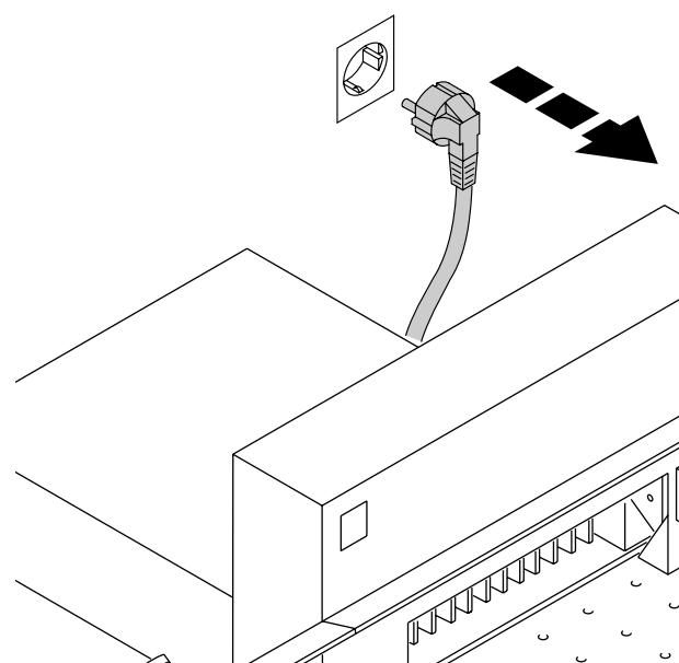
Disconnect from the mains before starting any service work or before removing the panels!
