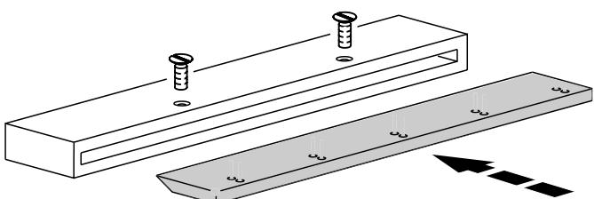
Place the blade into the blade carrier and screw it into place.
