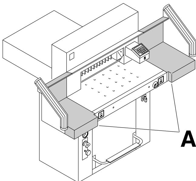
The machine is delivered ready for operation. Side tables (A), left and right are available as an option. Assembly instructions are included.
