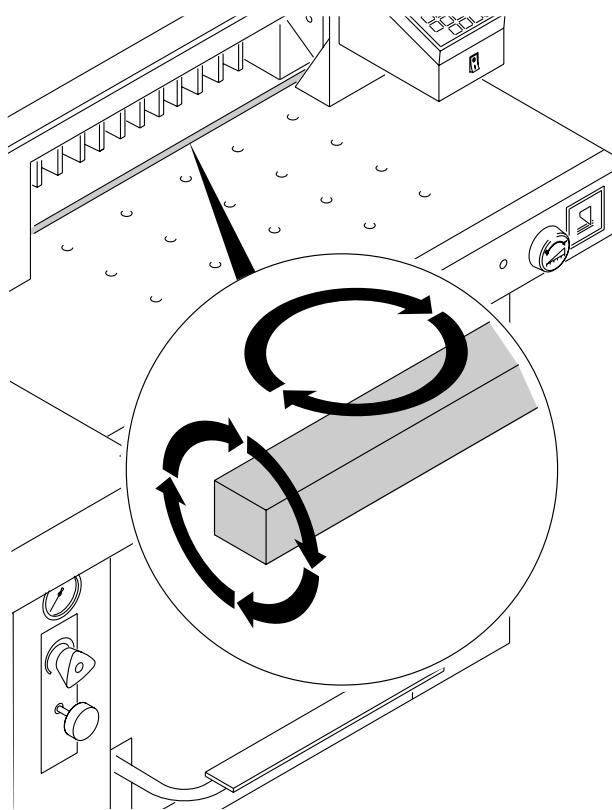
... or turn / replace the cutting stick (**B**). (See page 27 "Blade and cutting stick replacement").
