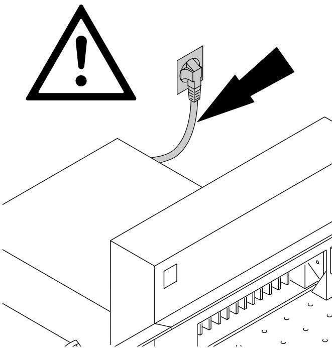
Protect mains cable against heat, oil and sharp edges!
