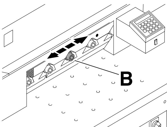
Push the blade and screw (**B**) as far as possible to the left or right and then centralize them. → The blade must rest on the cutting stick.
