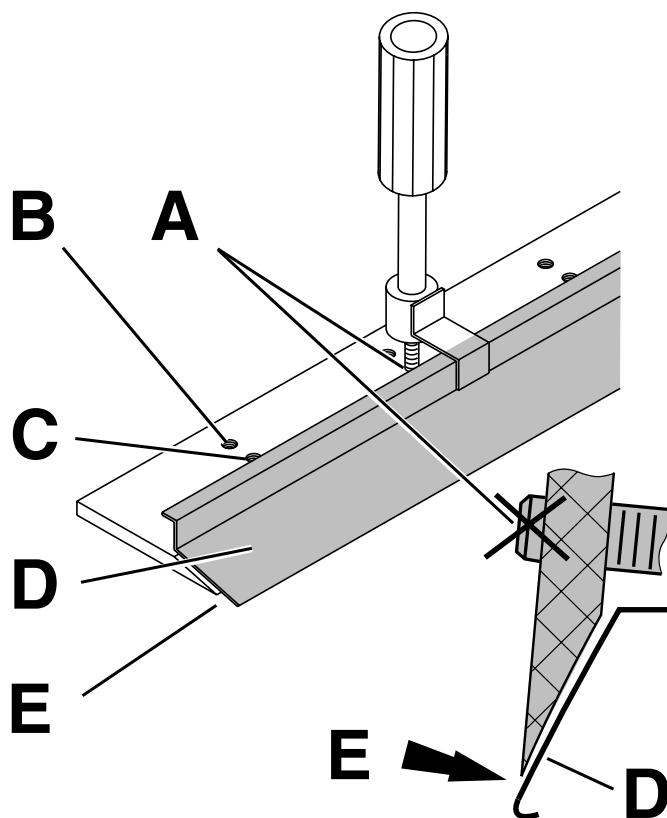
Take the exchange blade carefully out of the blade box and screw it to the blade changing tool (**D**).
