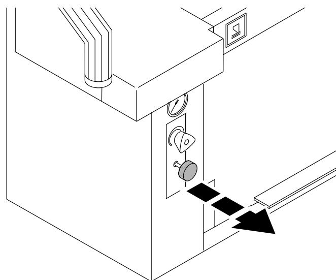
Pull out blade locking key → blade moves to the top.
