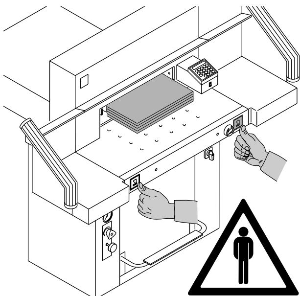
The machine is designed for cutting stacks of paper to a specified size. This machine is constructed for "one-man operation" only!
