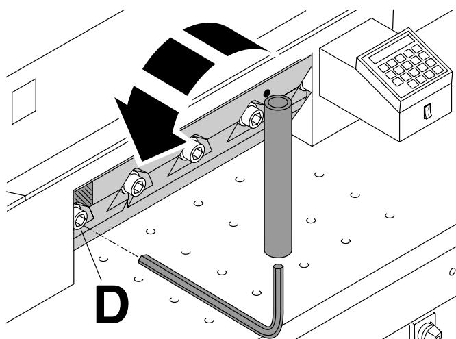
Remove the left screw (D), using the extension.
