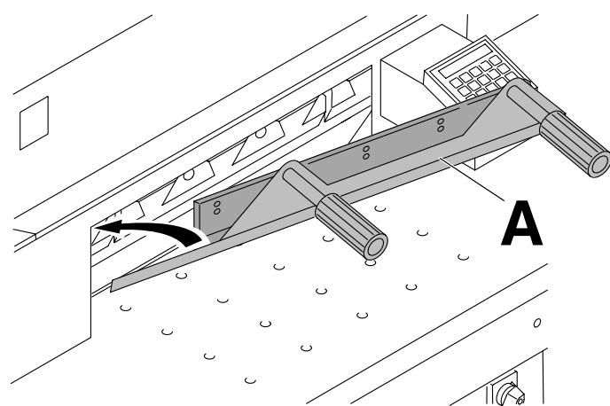
Mount the blade with the blade changing tool (**A**) ...
