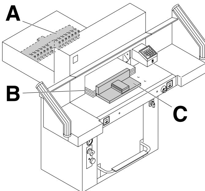
Position the paper on the backgauge (A) and side lays left or right (B). To move paper stacks, please use the paper knock-up block (C) provided.
