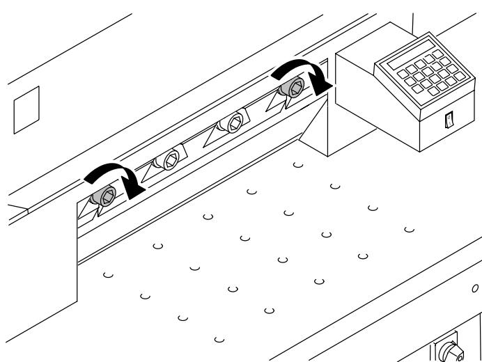
Slightly screw in outer screws.
