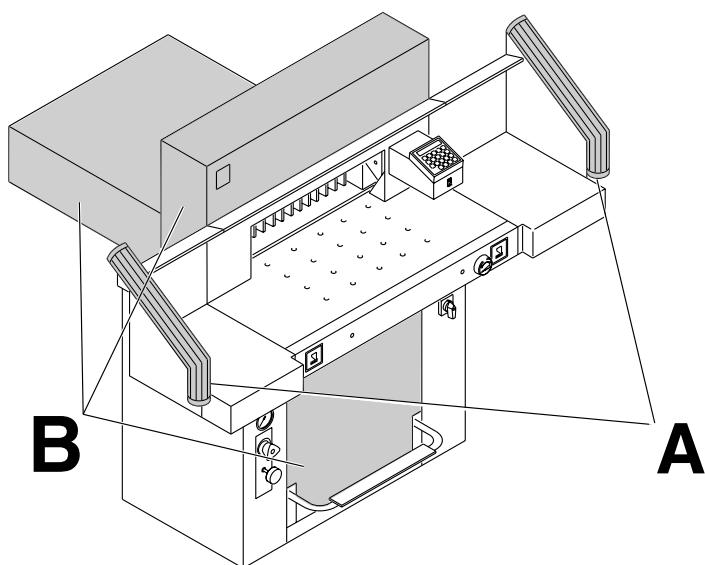
All components which could endanger the operator are covered by a guard (B)!
