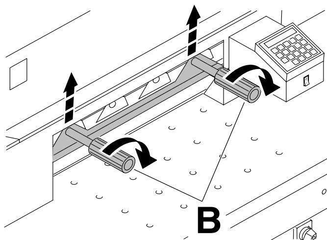
... and tighten with screws (**B**) in upper position.
