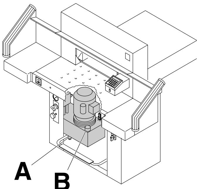
Grease and oil the machine according to the lubrication diagram after 1000 operating hours or once a year. If the machine is subject to excessive load then twice a year.
