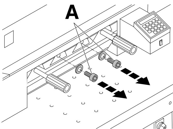
Remove remaining two screws (A).
