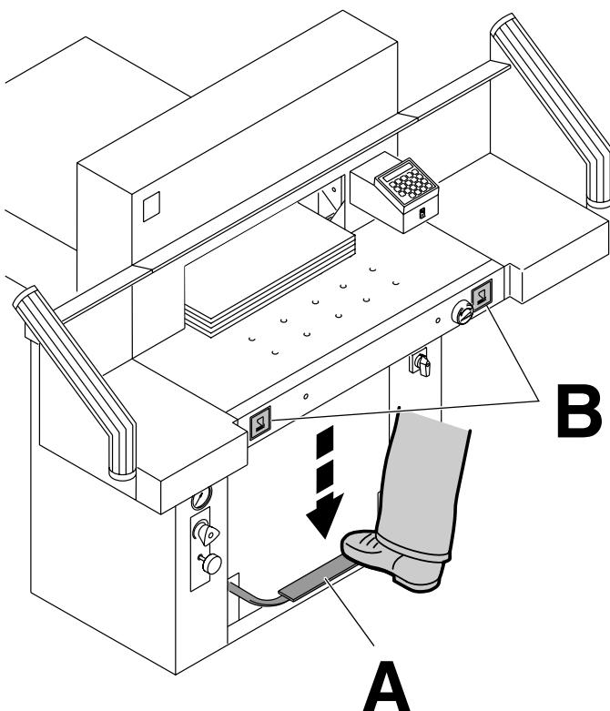
The clamp moves automatically when cutting is activated. The paper can be pressed in advance, with the foot pedal (**A**). Cutting is activated by pressing both buttons (**B**) on the front table.
