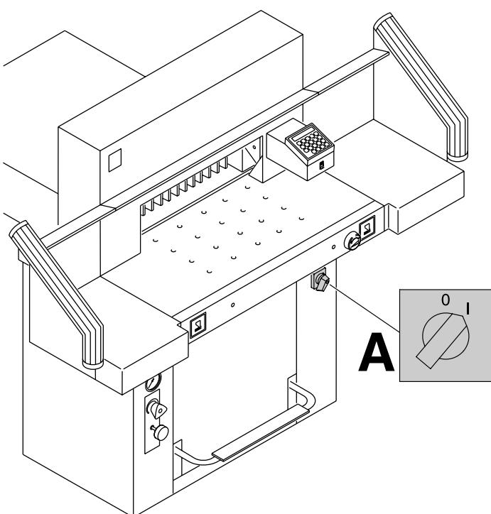
Paper cutting test. If the last sheet or several sheets are not completely cut, gradually turn the knob for blade depth adjustment (**A**) 1/6 turn to the left until the paper is cut along the entire length. Do not set too low as blade will soon become blunt.
