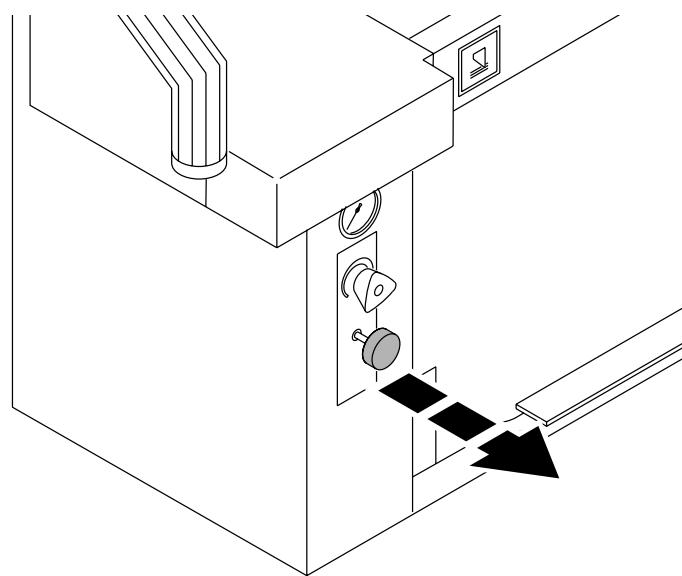
Pull out blade locking key → blade moves to the top.
