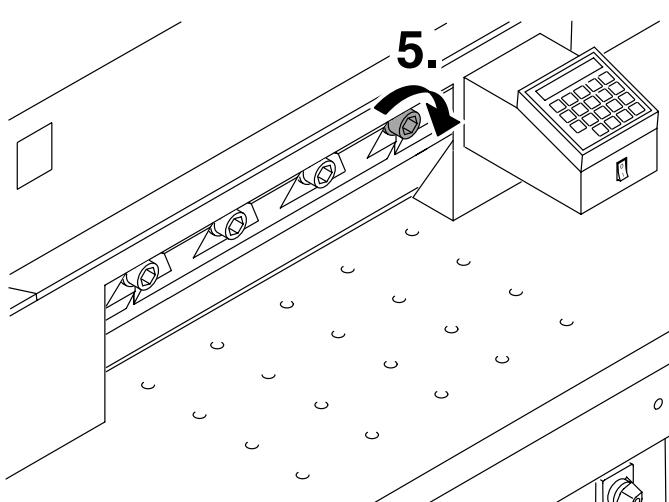
Tighten the screw which is visible at the right.
